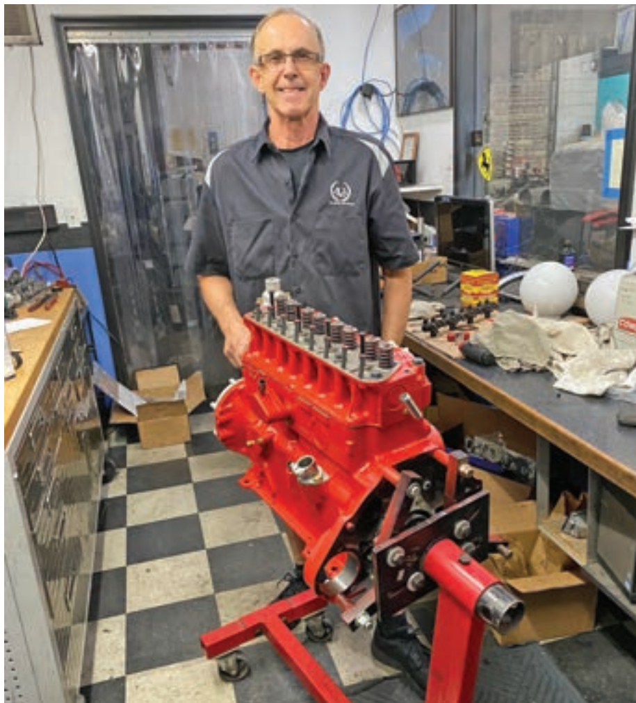
Robert Marcello, owner of Sacramento Volvo Service, and his team rebuilt the engine, including replacing the cracked head. They also made a number of improvements, such as upgrading the stock Bosch D-Jetronic fuel injection to a Holley Sniper EFI system.
